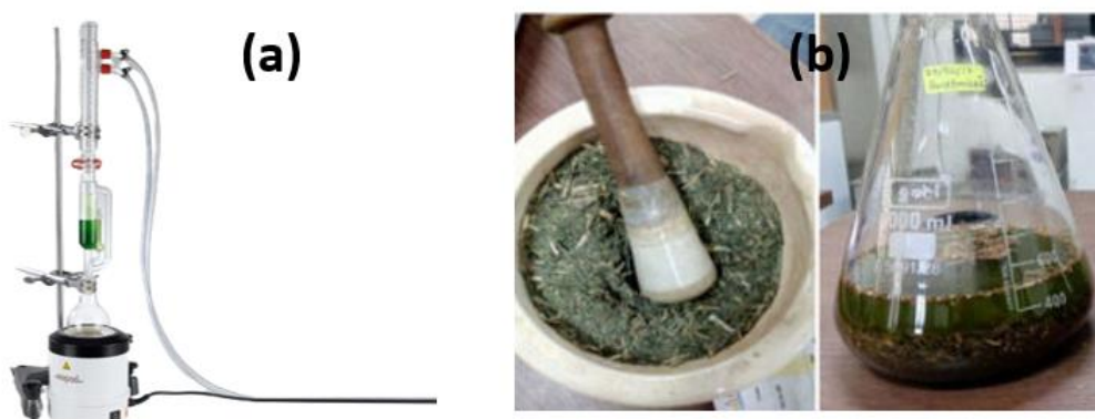
Fig. 2. Extraction of Mullein and Caralluma tuberculata leaves (a) Soxhlet Extraction (b) Maceration
