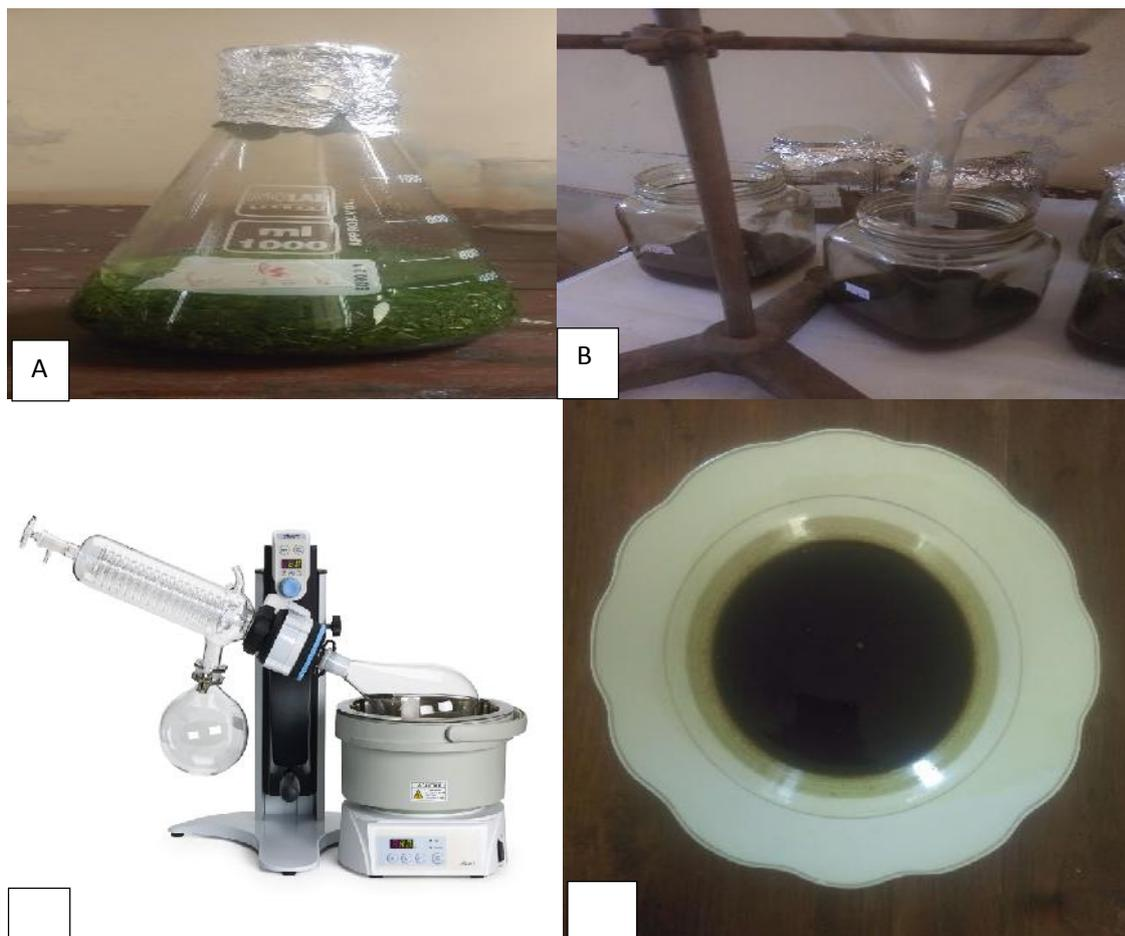
Figure 2: Preparation of plants extracts, A: Leaves with solvent; B: Filtered extract; C: Rotary evaporator (source: appletonwoods.co.uk. 2021);D: Crude extract.
