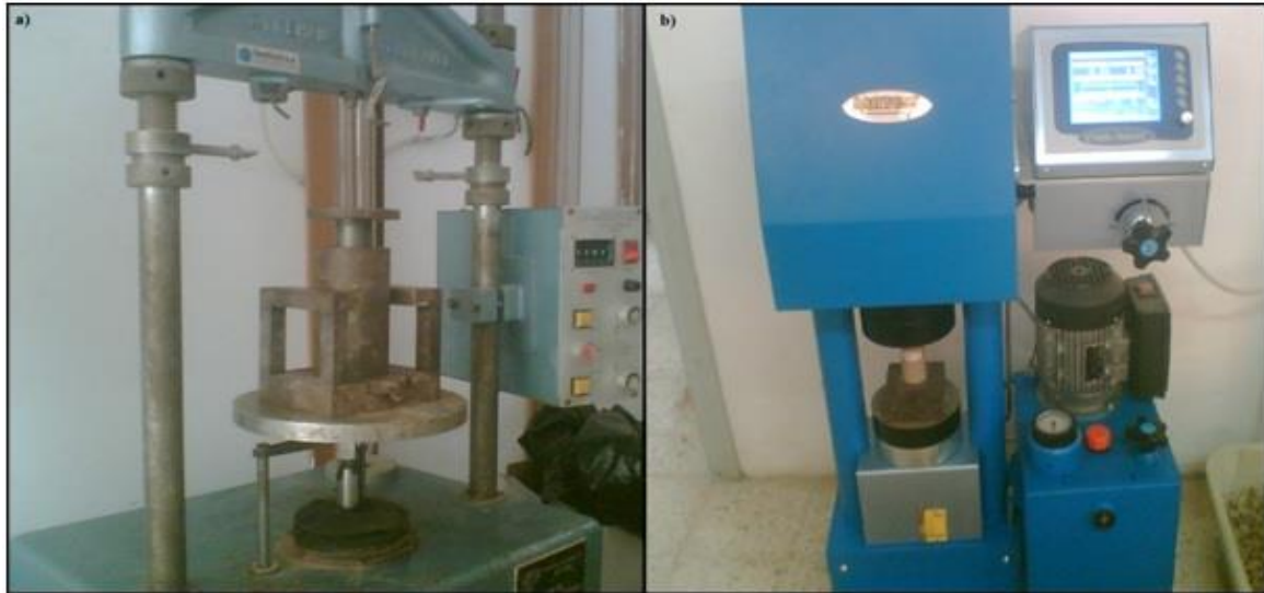
Figure 2: (a): Triaxial press (pressure = 40 Bar); (b): Triaxial compression test for each specimen
