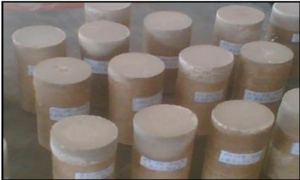
Figure 3. Standard cylindrical specimens of Solidified/Stabilized sludge
